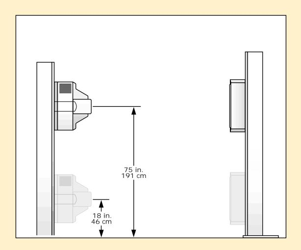
The DR 5100 system offers a vertical range of motion of 18 to 75 inches (46 to 191 cm) and servo-linked chest and tube stand.
